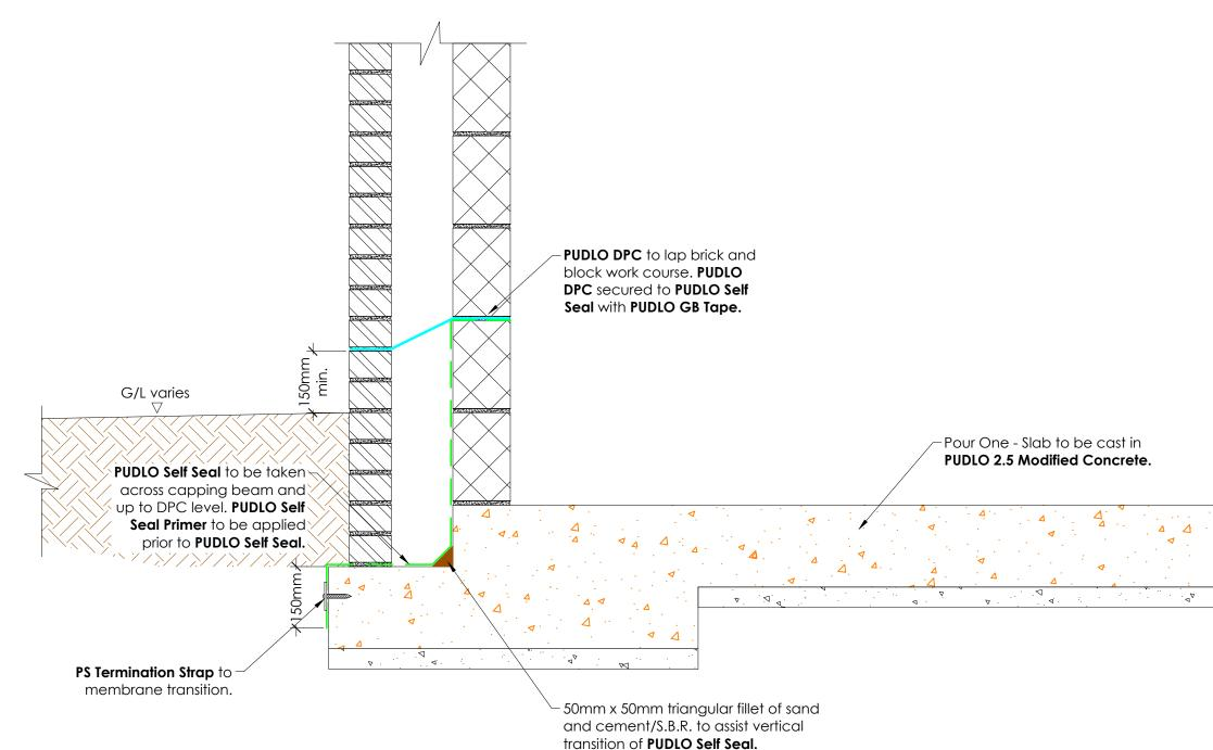
This PUDLO detail is to assist with the installation of its products. The detail shows how PUDLO 2.5 Modified Concrete and how PUDLO ancillaries are to be installed. For site specific details and confirmation on extent of where PUDLO 2.5 Modified Concrete is used i.e. Overlay drawings, must be confirmed by structural engineers/contractor. Individual/Company responsibility for design of the structure must ensure that details shown on PUDLO drawings match the latest construction issue drawings.
