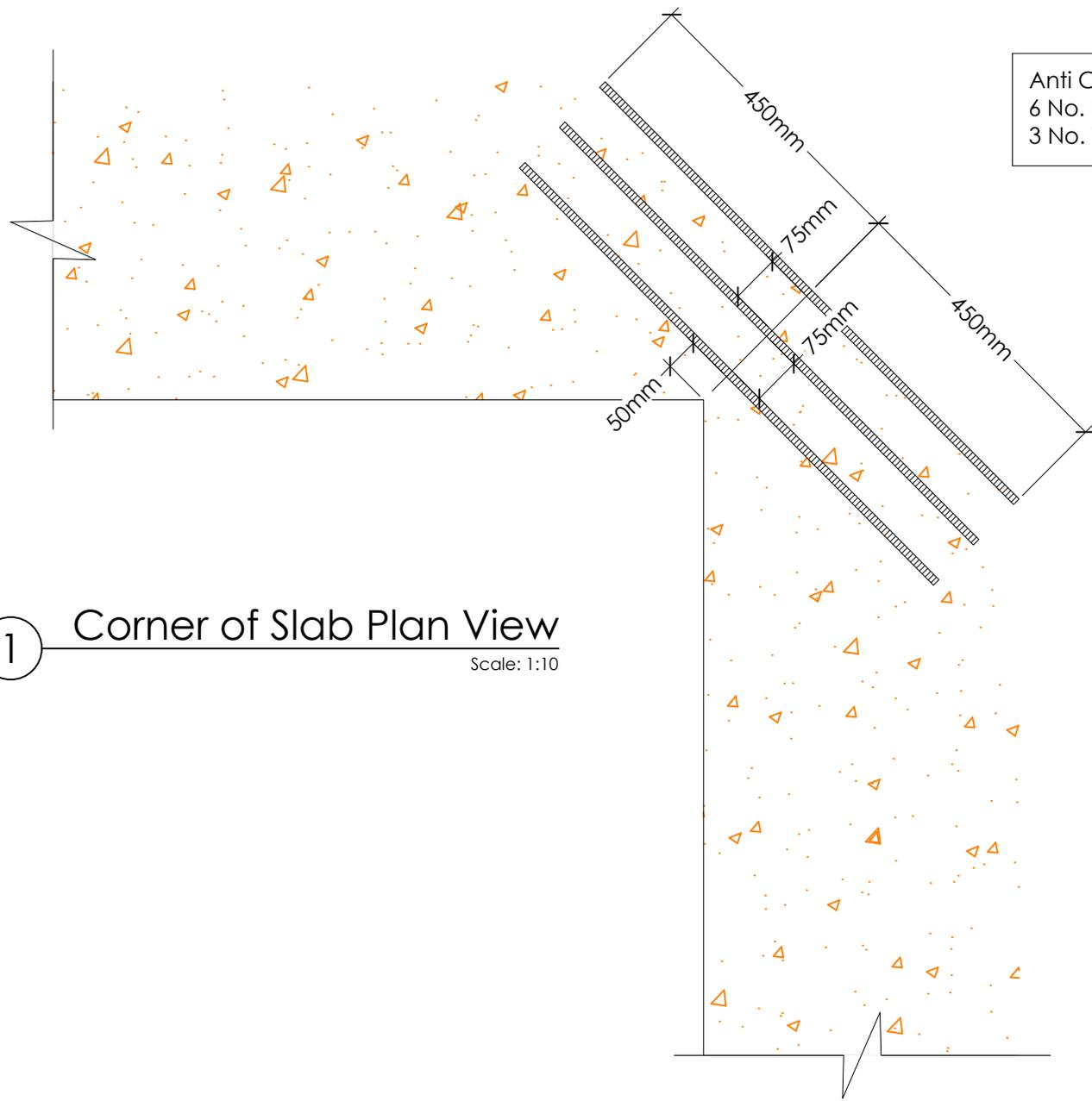
Anti Crack Reinforcement
