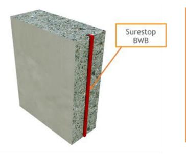
Surestop BWB is supplied in 25mm x 20mm x 5m coils, in boxes ( $6 \times 5$  metre rolls per box). For fixing instructions please refer to:
