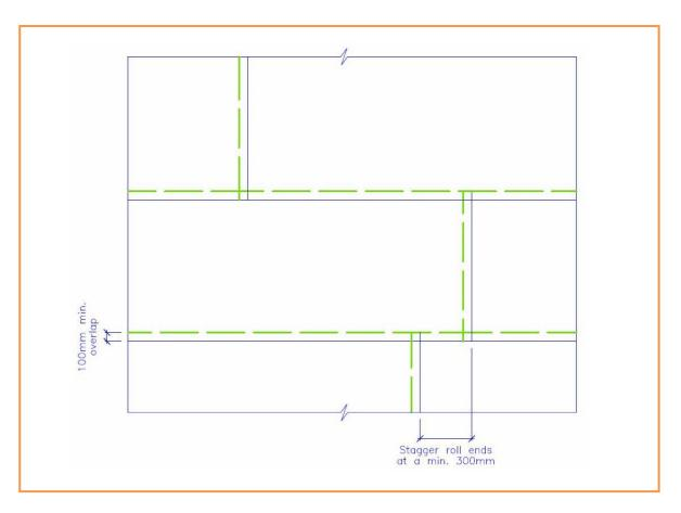
If the concrete base is poured in sections, PUDLO Membrane BW should extend a minimum of 300mm beyond the slab edge. This allows for the membrane to be properly overlapped (see below).
