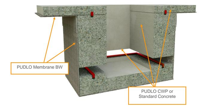
*PUDLO Membrane BW* should be placed on vertical surfaces, on the substrate below the lift pit base to form a continuous seal around the lift pit box. If the vertical soil is smooth and stable, then the *PUDLO Membrane BW* may be installed directly against the soil.
