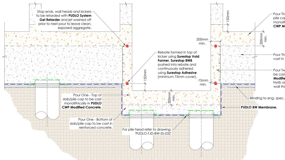
This PUDLO detail is to assist with the installation of its products. The detail shows how PUDLO CWP Modified Concrete and how PUDLO ancillaries are to be installed. For site specific details and confirmation on extent of where PUDLO CWP Modified Concrete is used i.e. Overlay drawings, must be confirmed by structural engineers/contractor. Individual/Company responsibility for design of the structure must ensure that details shown on PUDLO drawings match the latest construction issue drawings
