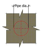
**PUDLO BW Membrane** 'cross-cut' to diameter of service. PUDLO BW Membrane to be passed over pipe.
