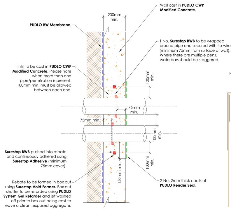
N.A. - Box out service penetrations are not acceptable in swimming pool construction.
