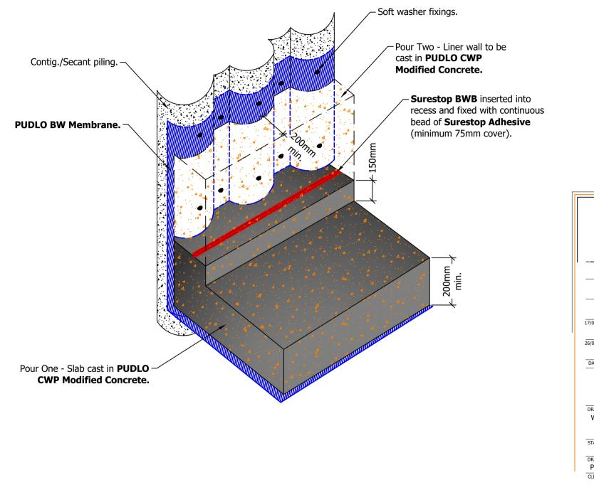
This PUDLO detail is to assist with the installation of its products. The detail shows PUDLO CWP Modified Concrete and how PUDLO System accessories are to be installed. For site specific details and confirmation on extent of where PUDLO CWP Modified Concrete is used i.e. Overlay drawings, must be confirmed by structural engineers/contractor. Individual/Company responsibility for design of the structure must ensure that details shown on PUDLO drawings match the latest construction issue designs.
