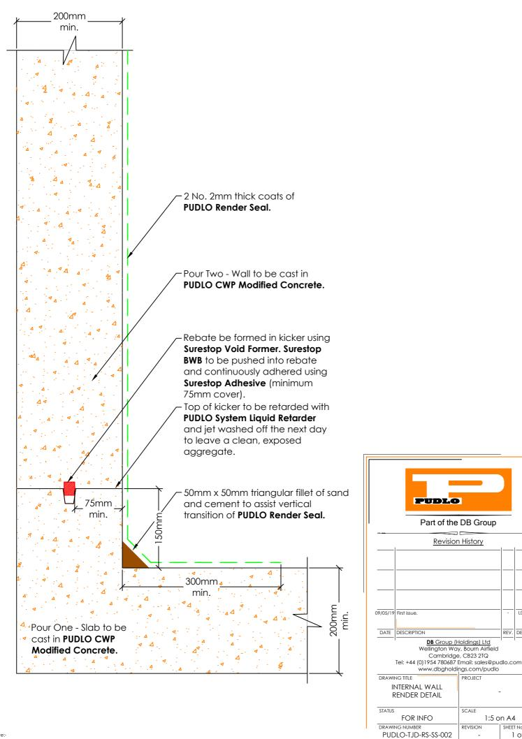
This PUDLO detail is to assist with the installation of its products. The detail shows how PUDLO CWP Modified Concrete and how PUDLO ancillaries are to be installed. For site specific details and confirmation on extent of where PUDLO CWP Modified Concrete is used i.e. Overlay drawings, must be confirmed by structural engineers/contractor. Individual/Company responsibility for design of the structure must ensure that details shown on PUDLO drawings match the latest construction issue drawinas
