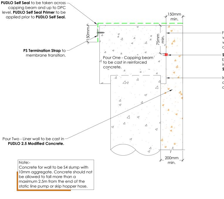
Face of capping beam to be retarded with PUDLO System Gel Retarder and jet washed off prior to wall pour to leave a clean, exposed aggregate.
